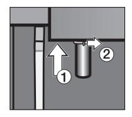
■ Push the froth dispenser into the machine from below, ①, and turn the cover above the spout to the right, ②.
